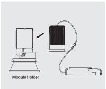
2. Attach module to module holder 3. Adjust the angle required. with spring clip and connect module to driver.
