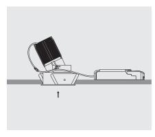
4. Gently insert module holder from the bottom of the fixture frame to complete installation.
