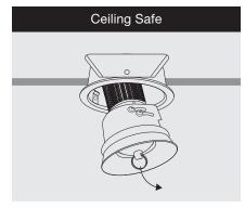
Remove module holder with suction cup for LED module replacement / maintenance.
